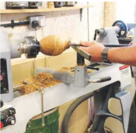
STEP 14. Your stance is very important when using a hollowing tool. Swivelling the head on the lathe means that you haven't got to lean over the bed, which could make the whole process rather uncomfortable
